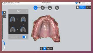
Ensure the full arch information is fully recorded for denture production in Denture Mode.
