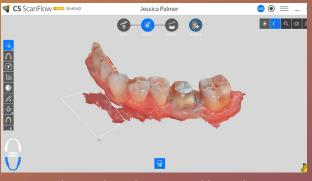
Cut several areas from the scan and keep the cutting tool activated while rotating the digital impression.
